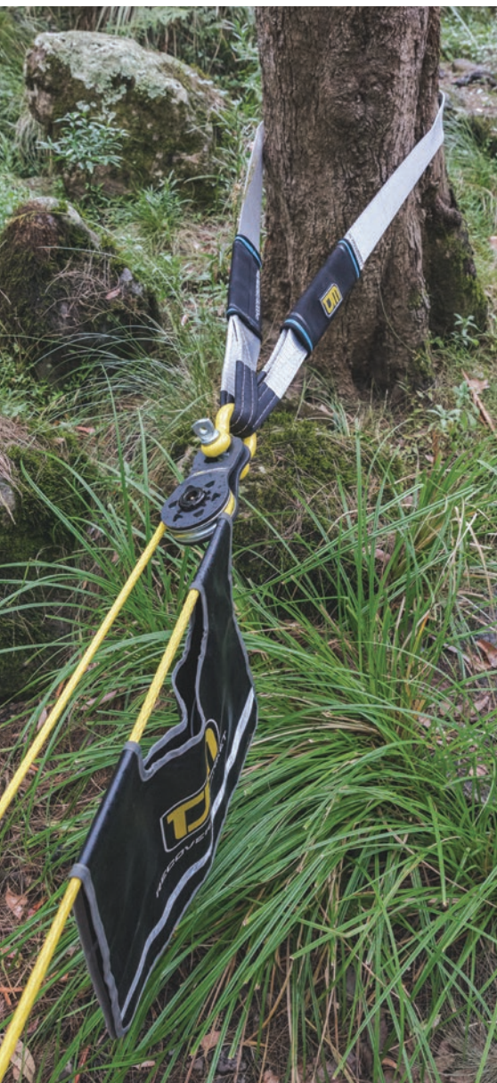
Using a Tree Trunk Protector, Bow Shackle and a Snatch Block from the TJM Large Recovery Kit in a double-line winch recovery.
