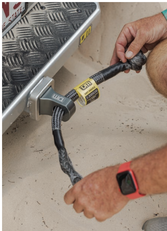
A TJM soft shackle provides a simpler and safer means of vehicle recovery.
