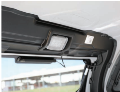
Clockwise: LED Interior Light. No-drill C-clamp mounting system.
