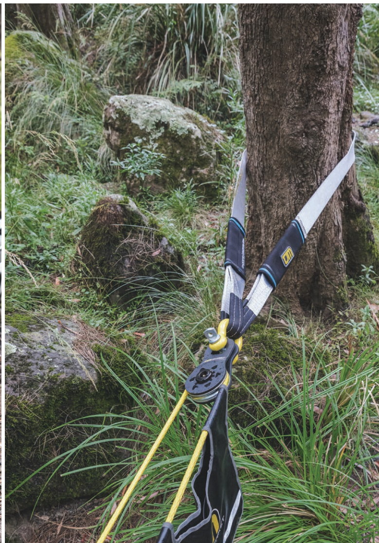
Using a Tree Trunk Protector, Bow Shackle and a Snatch Block from the TJM Large Recovery Kit in a double-line winch recovery.
