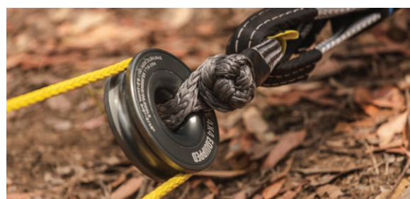
Using a Tree Trunk Protector, Bow Shackle and a Snatch Block from the TJM Large Recovery Kit in a double-line winch recovery.
