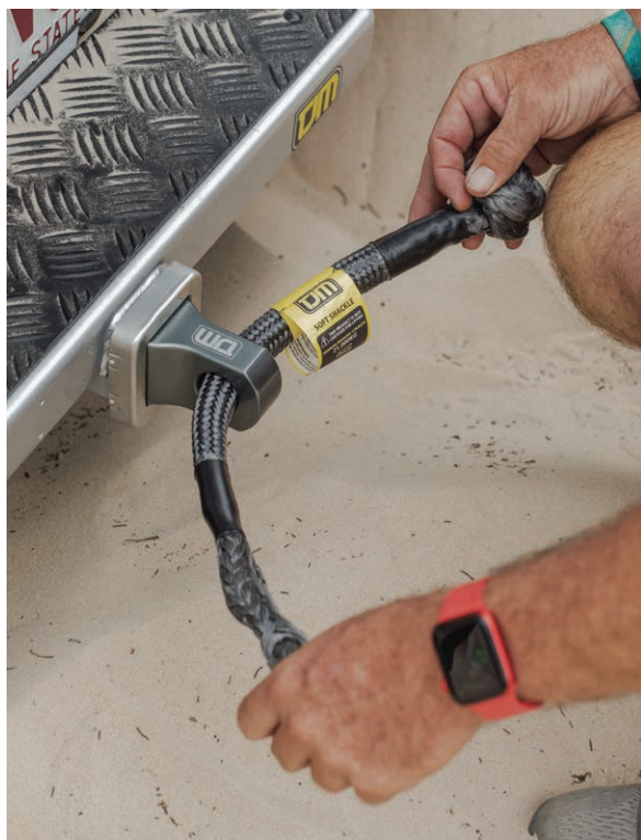
A TJM soft shackle provides a simpler and safer means of vehicle recovery.
