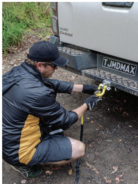
A TJM bow shackle can be used with a TJM Steel Recovery Hitch.
